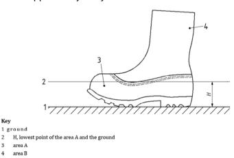
The materials of area A and B may be connected by stitching, welding or other suitable methods. When tested according to ISO 20344:2021, 5.25 the connection shall fulfil a strength of at least 10 N/mm.
